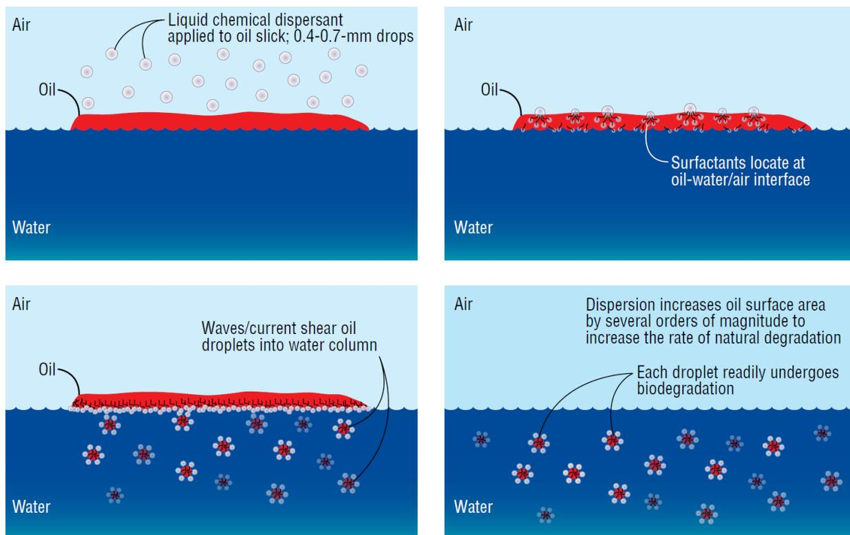
Figure 2. Schematic drawing illustrates the dispersion process.
