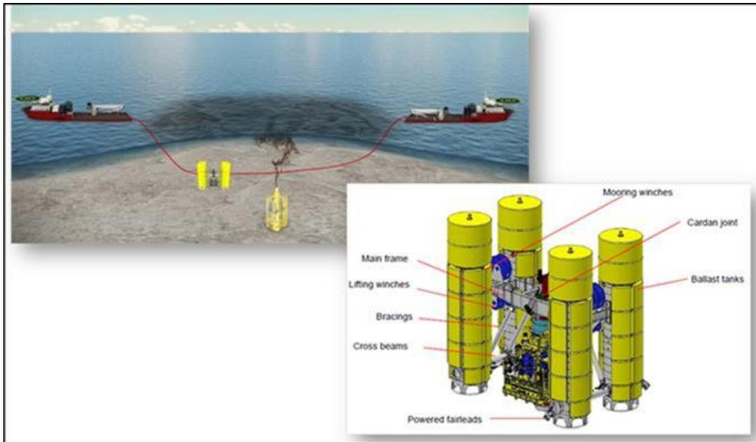
Figure 10. SWRP Offset Installation Equipment Concept
