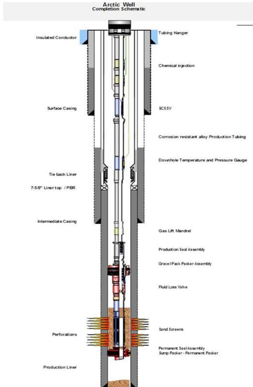
Figure 15. Example of an arctic well completion
