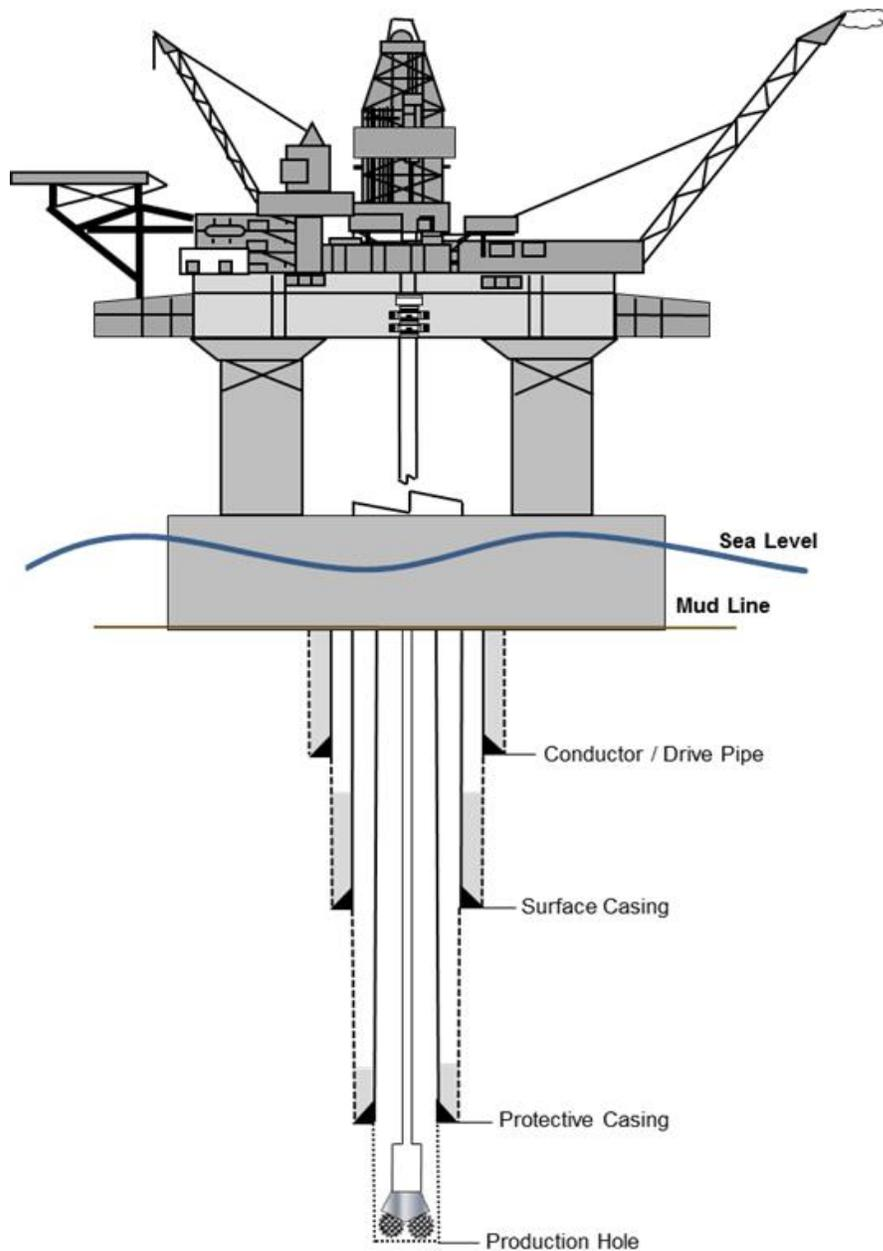
Figure 2. Schematic of a Surface Drill Well – Drilling Phase
