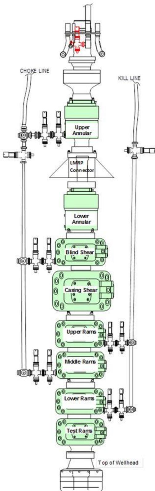
Figure 6b. Typical Subsea Blowout Preventer Stack (multiple redundancy)
