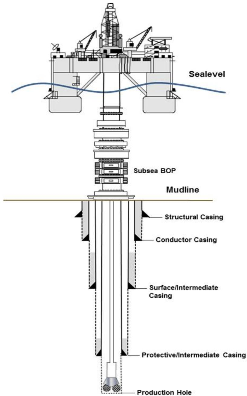
Figure 3. Schematic of a Subsea Drill Well – Drilling Phase
