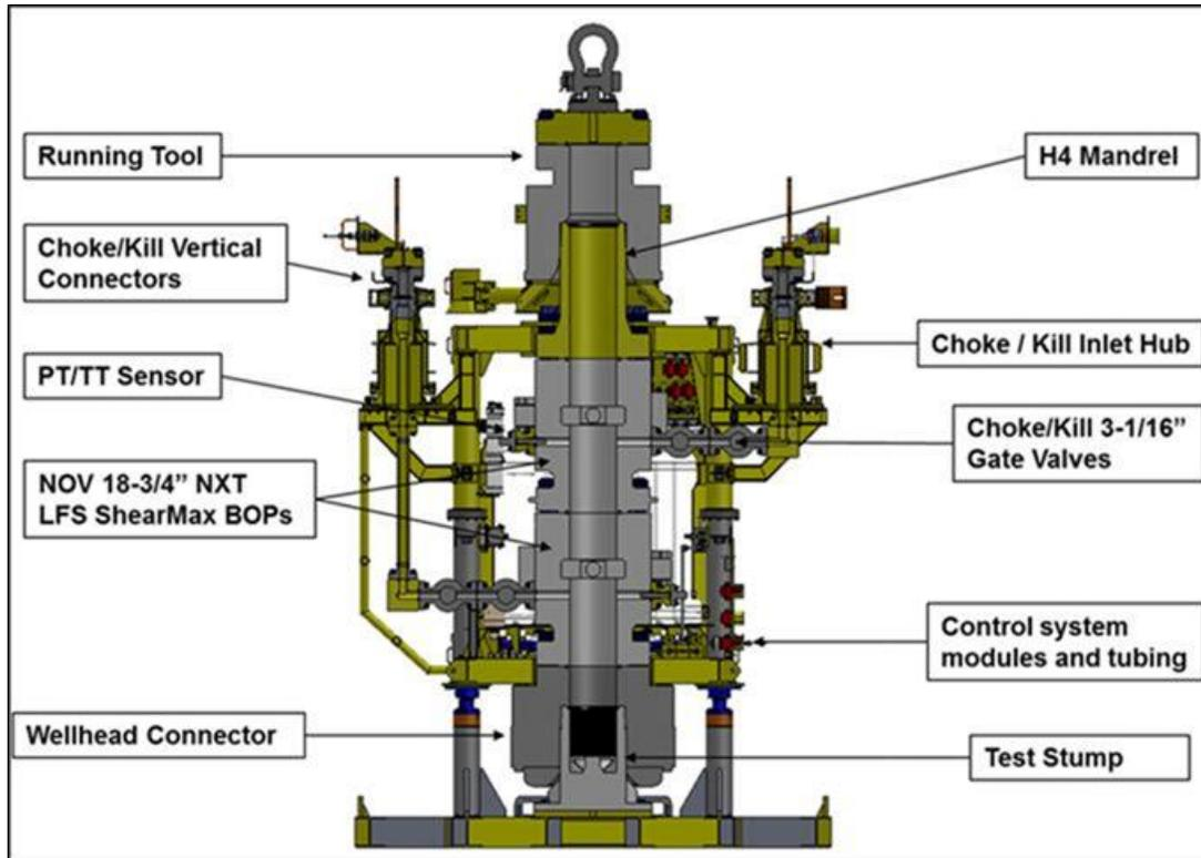
Figure 13. Internal View of a Subsea Shut-in Device
