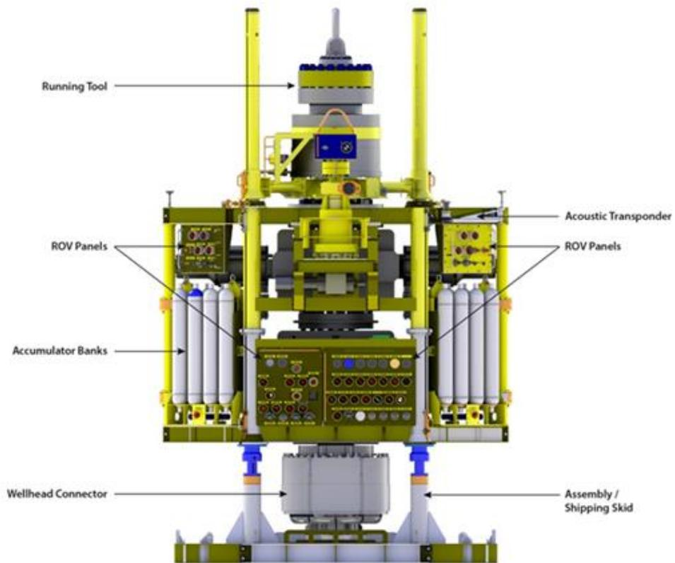
Figure 12. External View of a Subsea Shut-in Device
