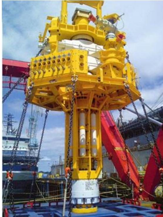
Figure 9. Capping Stack, Shell Arctic Capping Stack
