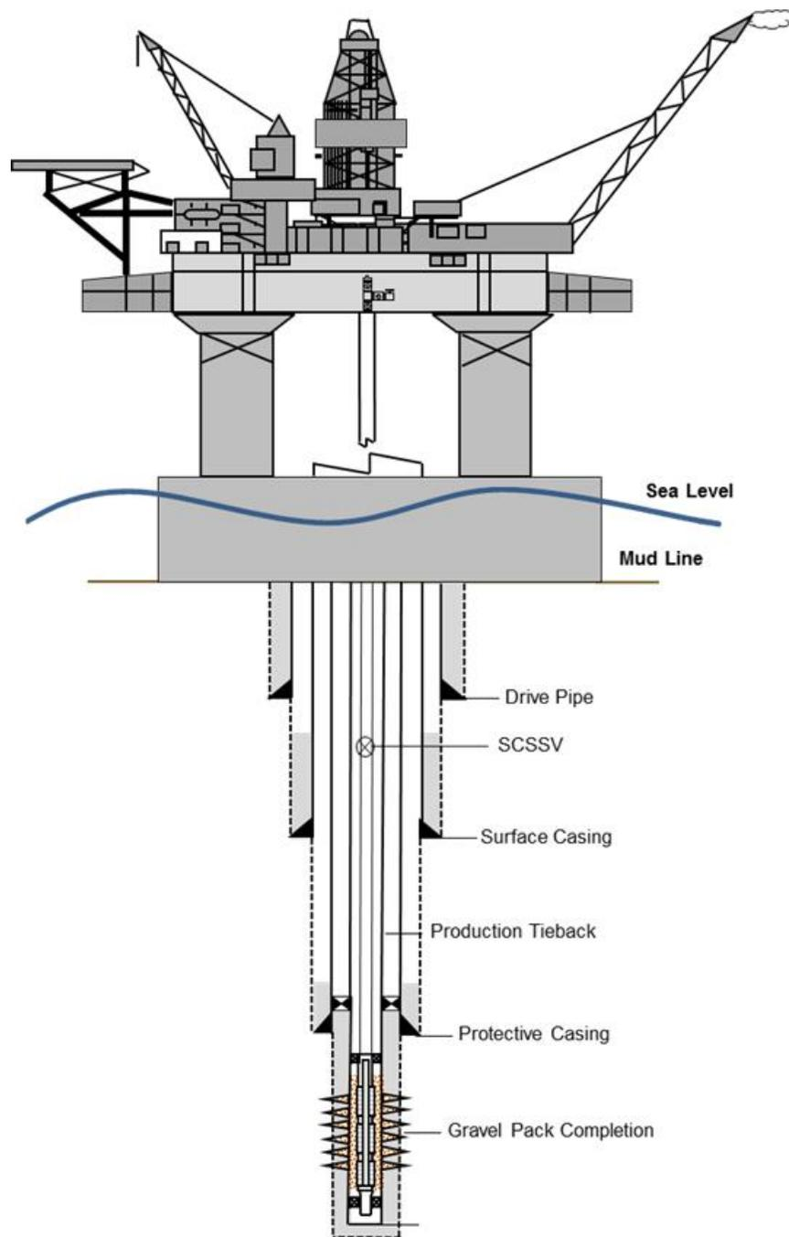
Figure 4. Schematic of a Surface Drill Well – Completion/Production Phase
