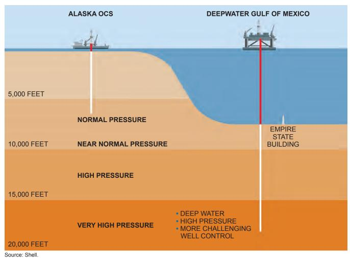
*Figure C-8.* Comparison of the Subsurface Environment of the U.S. Arctic Potential with the U.S. Deepwater Gulf of Mexico, for Offshore Exploration Drilling
