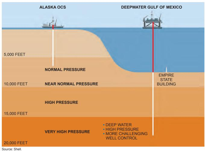
*Figure 4.* Comparison of the Subsurface Environment of the U.S. Arctic with the U.S. Deepwater Gulf of Mexico, for Offshore Exploration Drilling
