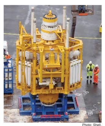
Figure 6. Subsea Isolation Device used for Drilling in the Kara Sea
