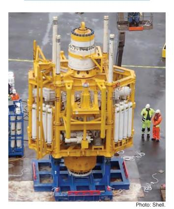
Figure C-13. Subsea Isolation Device Used for Drilling in the Kara Sea
