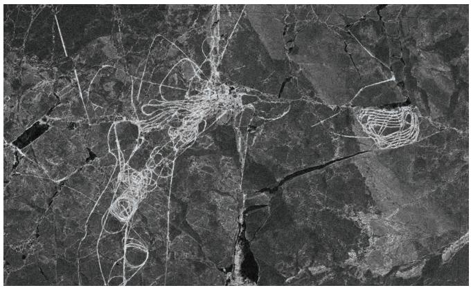
Photo: COSMO-SkyMed Image ©ASI (2017). All rights reserved. Processed and delivered by KSAT. Figure C-6. Cosmo Sky-Med Satellite Image Overlooking Test Area. Visible Tracks from Ice Management
